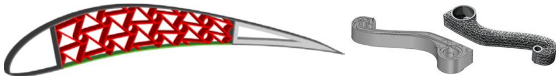
Fig.1: auxetic actuated wingbox (left) and AM optimized parts (Airbus, right)
