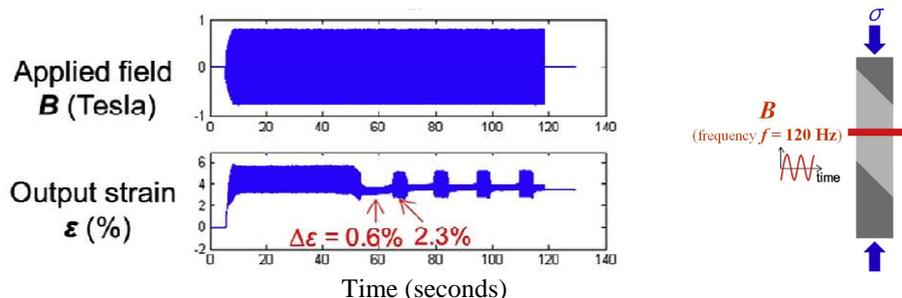
“Autonomous” (self-organized) oscillation occurred in a classical active system (The cyclic oscillation of strain amplitude of a Magnetic Shape Memory Alloy under a given magnetic field developed automatically) <sup>[4, 5]</sup>.
