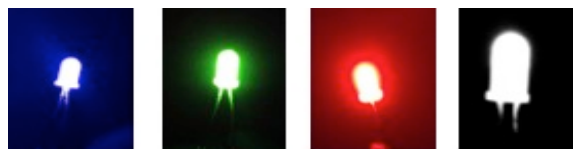
Figure. Near-UV LEDs coated with luminescent polymers.
